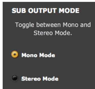
The **2Way Advanced 21** plugin supports mixing of two output channels, allowing this plugin to be used in “2.1” applications where a mono subwoofer signal is derived from a stereo signal. To access this selection, click on the **System Settings** tab.
