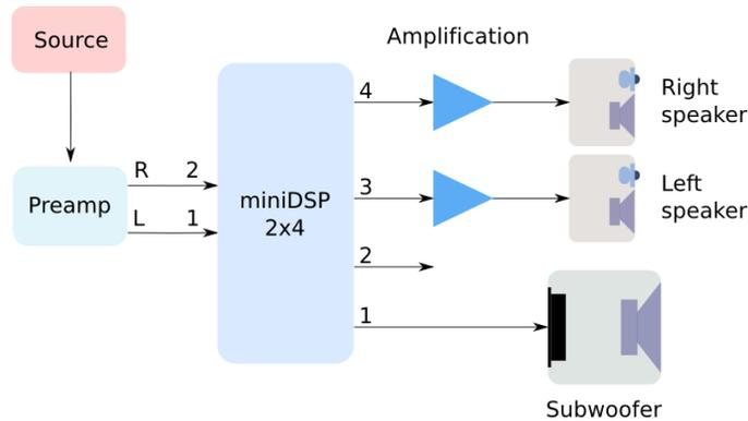
To accomplish this configuration, use the matrix mixer to mix input channels 1 and 2 to output 1, and to send input 1 to output 3, and input 2 to output 4:
