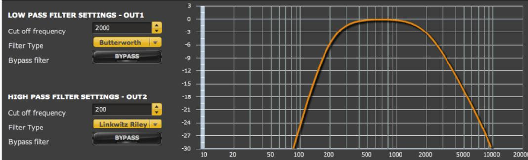
High pass and low pass filters are a subset of crossover functionality. These blocks have a single input and a single output. Each filter can be individually set to one of the available filter types, or bypassed. The filter types are:
