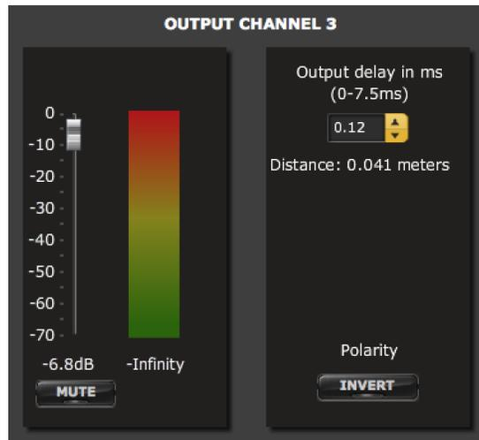
Each output channel has a gain control, together with a level meter (active while the plugin is in online mode), adjustable delay, a mute button and a button for polarity inversion.
