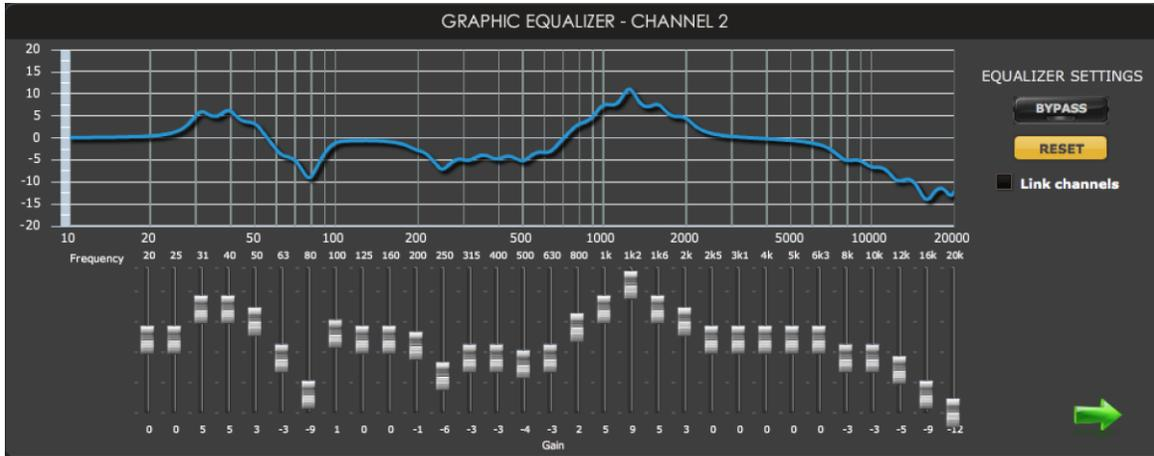
The graphic equalizer block (GEQ) presents a 31-band, 1/3<sup>rd</sup> octave EQ, similar to a “traditional” analog EQ. The top section shows the overall response curve of all EQ bands. Hovering the mouse over the curve brings up an overlay with the frequency and gain at that frequency.
