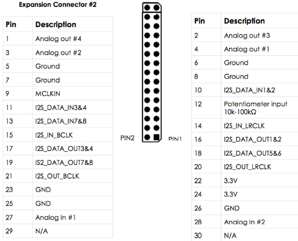
I2S, also known as Inter IC Sound, is an electrical serial bus used to interface digital audio devices at the chip and circuit board level. Note that I2S is not a “plug and play” protocol, and requires attention to technical details such as clocking and wire layout. It is a solution that we make available for *advanced* DIYers with suitable knowledge, skills and measurement equipment to use it.
