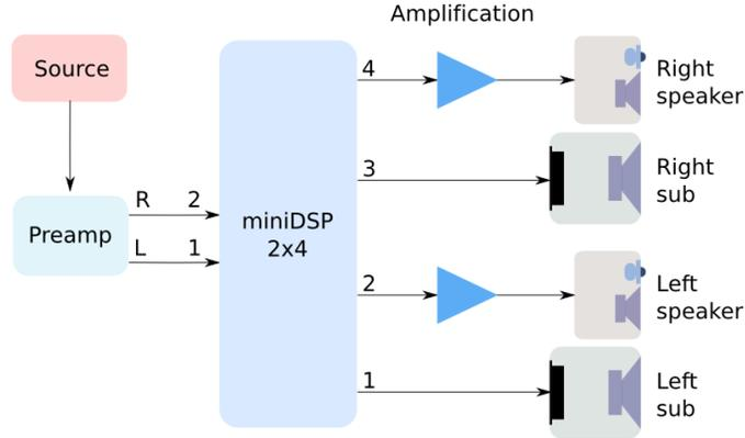
To accomplish this configuration, use the matrix mixer to send input channel 1 to outputs 1 and 2, and input channel 2 to outputs 3 and 4:
