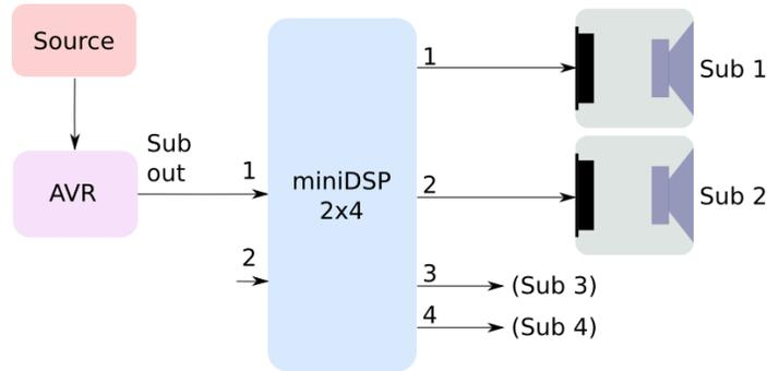
To accomplish this configuration, the routing matrix sends input channel 1 to all four output channels:
