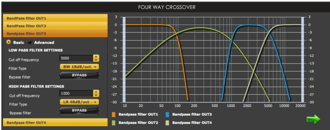
In the miniDSP 2x4 plugins, each output channel has a high pass filter and a low pass filter, each of which can be set to one of a range of filter types and slopes, or individually bypassed. Clicking on the bars labeled “CH1 Bandpass Filter OUT1,” and so on displays the filter parameters for that output channel.
