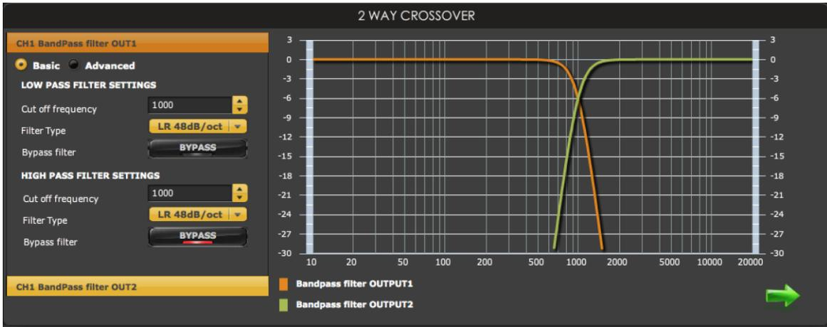
Crossovers “split” the frequency band to send to different drivers. In a two-way loudspeaker, for example, a *low pass* filter is used to remove high frequencies from the signal sent to the woofer, and a *high pass* filter is used to remove low frequencies from the signal sent to the tweeter. The above screenshot shows a two-way crossover. In a four-way crossover, the signal is split into four frequency bands:
