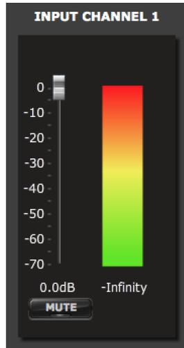
Each input channel has a gain control, together with a level meter (active while the plugin is in online mode), and a mute button.
