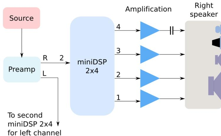
**[2x4 Advanced](#)** The new **2x4** crossover plugin provides parametric EQ on both inputs and on all four outputs, fully independent crossovers/filters with a wide range of filter slopes (up to 48 dB/octave) on all four outputs, and a matrix mixer. Three-way and four-way active loudspeakers are among the wide range of applications supported by this plugin. For more information, see the [datasheet](#).
