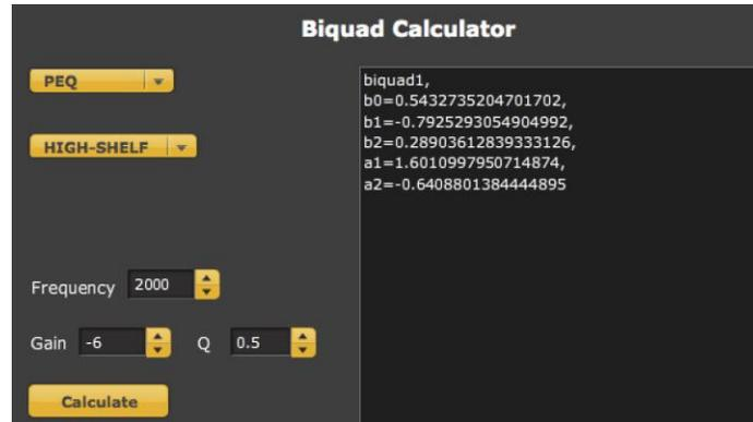
The calculator supports single parametric EQ bands, as shown in the above screenshot. To use the calculated biquad, simply copy the coefficients into the PEQ filter (set to Advanced mode) and click on the **Process** button.
