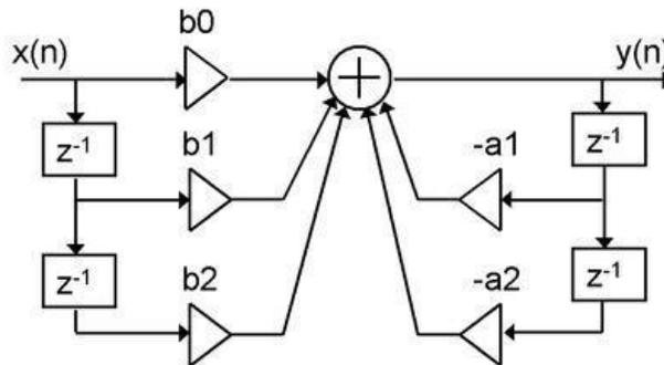
A single biquad like this can perform a great many functions, including all of the functions of a single parametric EQ filter, one 6 or 12 dB/octave high pass or low pass filter, and more. Biquads are combined in series (cascaded) to create more complex filters. The function that each biquad performs is determined by just five numbers:  $a_1$ ,  $a_2$ ,  $b_0$ ,  $b_1$ , and  $b_2$ . These numbers are called the *coefficients*.
