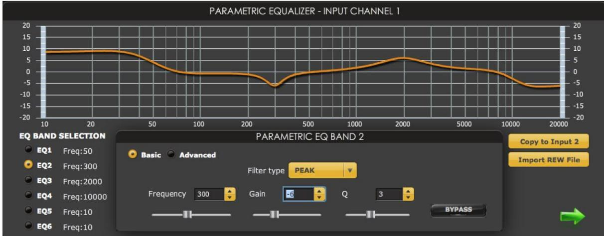
The parametric EQ (PEQ) block provides six parametric filters, each of which can be set for a peaking or notch filter, high shelf filter, and low shelf filter.
