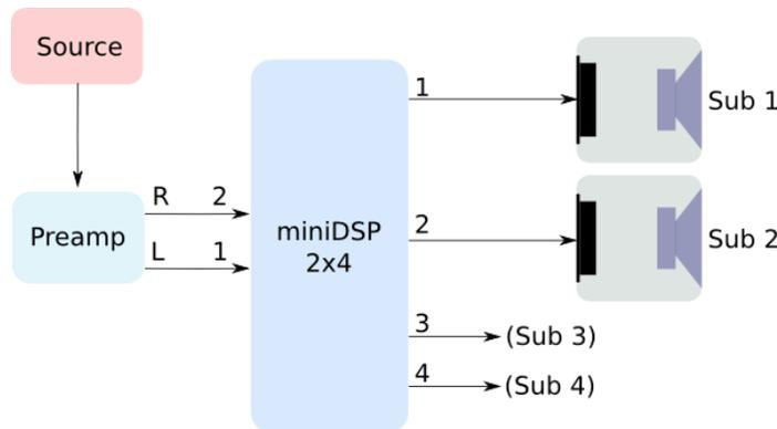
To accomplish this configuration, use the matrix mixer to mix both input channels to all four output channels:
